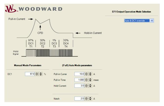
Auto mode The current profile is setup closed loop, current is actively controlled. There is Open Coil diagnostics and current compensation for (environmental) changes. There is no Closure Point Detection.
