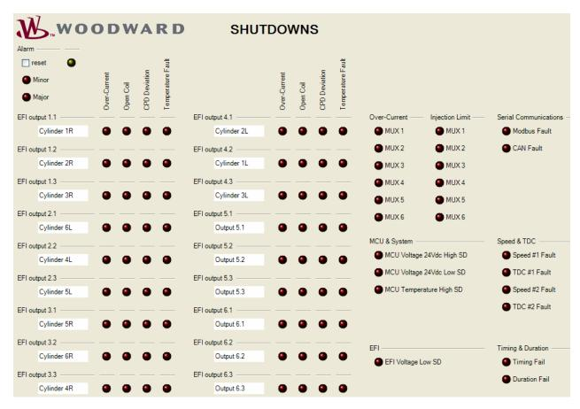
The Shutdowns page displays active and latched shutdowns with red LED's. Shutdowns will always stop the running operation mode of the EFI output.
