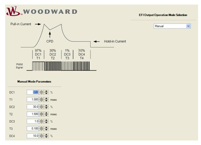
The required **EFI Output Operation Mode Selection** can be selected from the drop down list.
