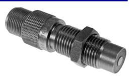
When a magnetic material (usually a gear tooth driven by the prime mover) passes through the magnetic field at the end of the magnetic pickup, a voltage is developed. The frequency of this voltage is translated by the speed control into a signal which accurately depicts the speed of the prime mover.
