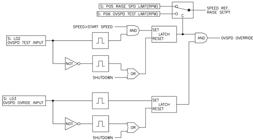
Figure 3-42. Overspeed test setting
