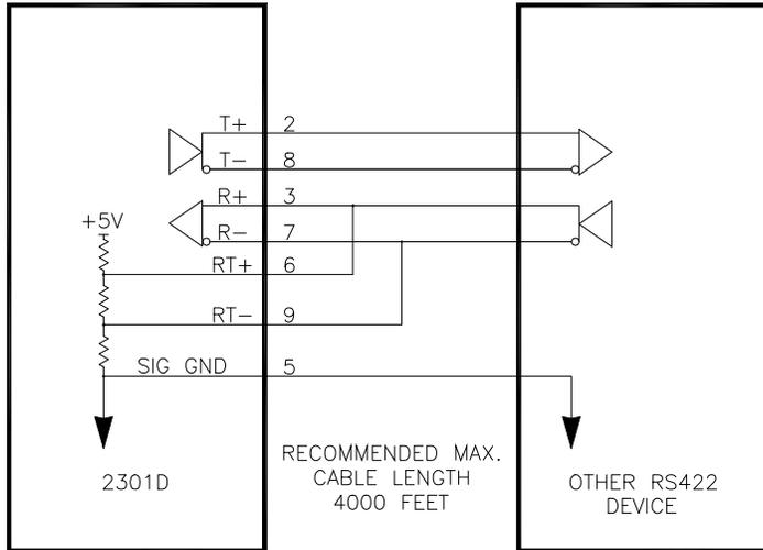
Figure 2-9. Typical RS-422 Communications Connections
