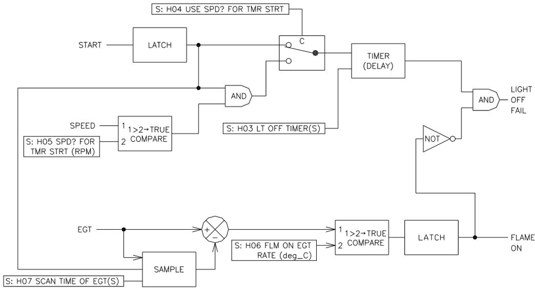
Figure 3-34 Light Off Fail Setting
