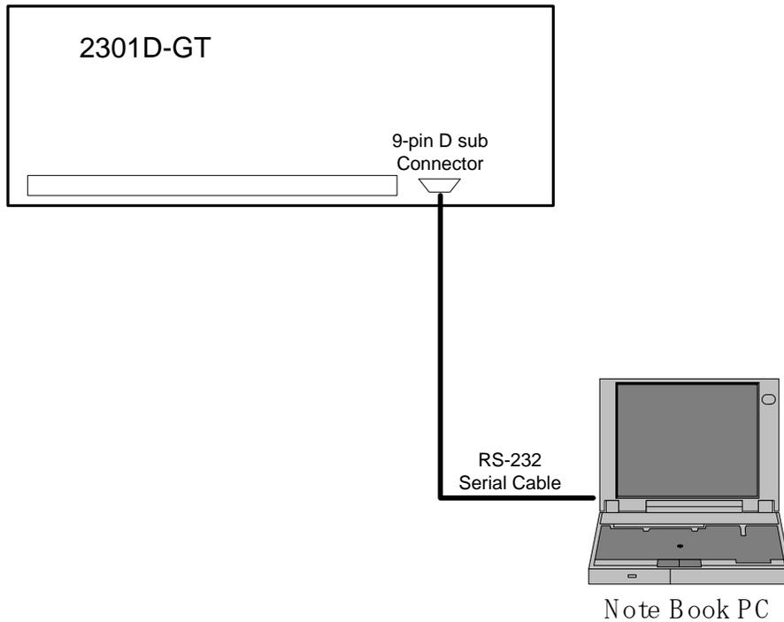
Figure 3-2. Connection between PC and 2301D-GT
