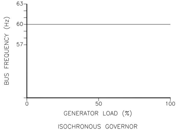
Figure 4-8. Isochronous Mode
