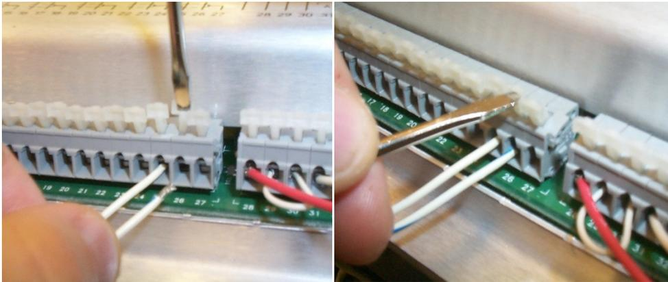
Figure 2-6. Installation of Wiring into Terminal
