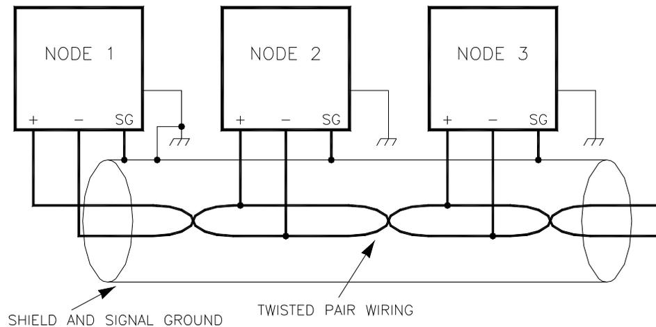
Figure 2-12. Alternate Multipoint Wiring Using Shielded Twisted-pair Cable without a Separate Signal Ground Wire
