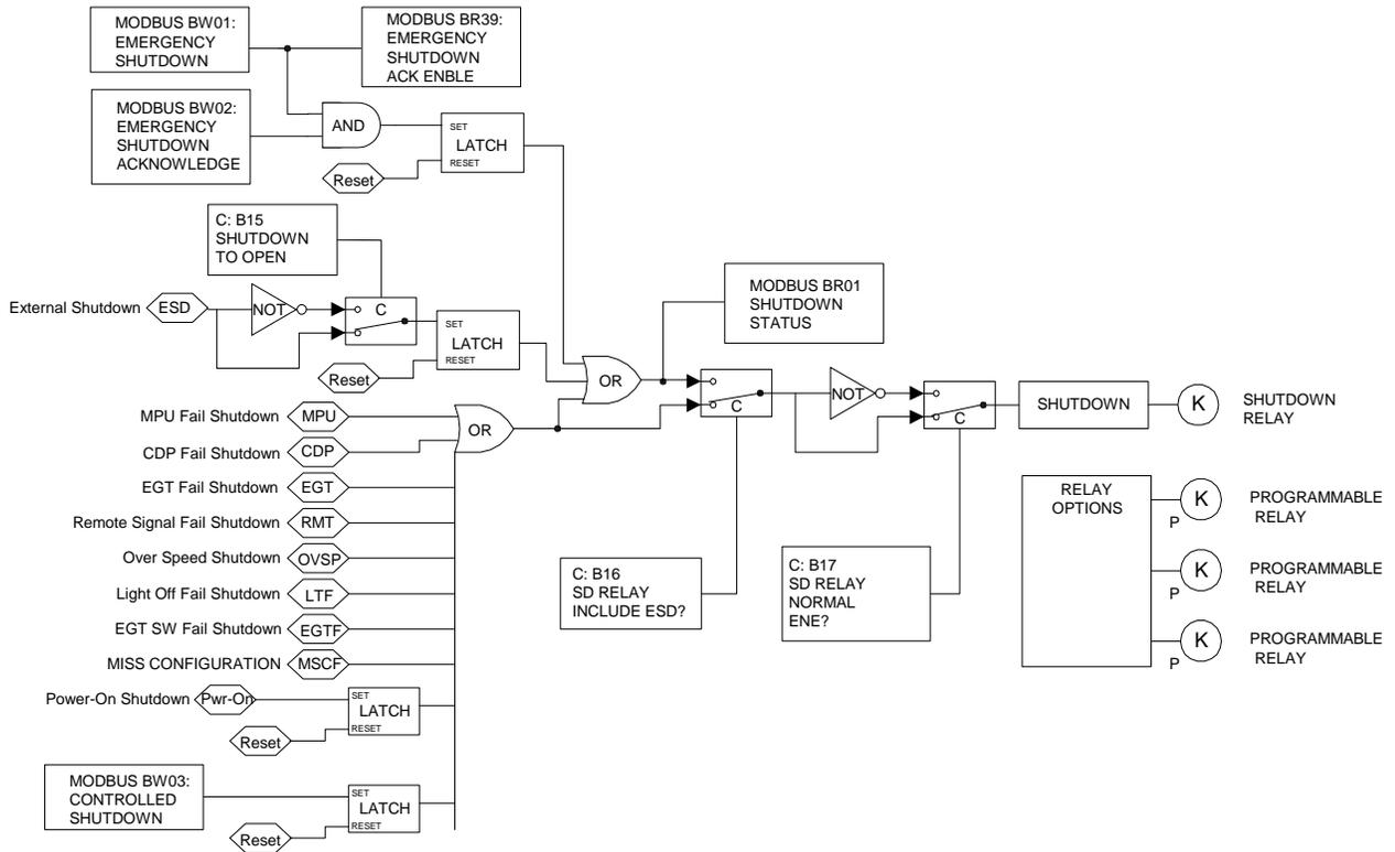
Figure 3-11. Shutdown Relay Configuration
