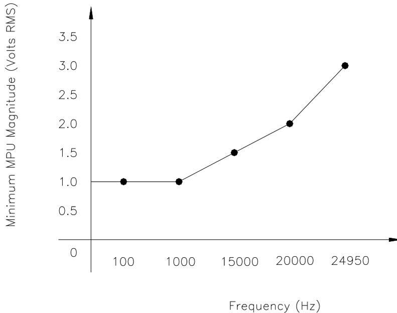
Figure 2-7. Minimum MPU Voltage
