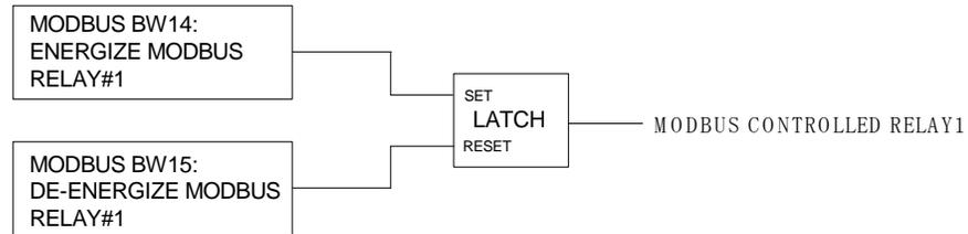
Figure 3-55. MODBUS CONTROLLED RELAY#1
