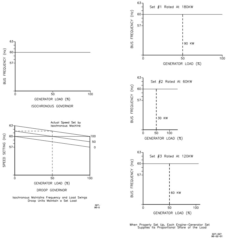
Figure 4-9. Droop/Isochronous Load Sharing
