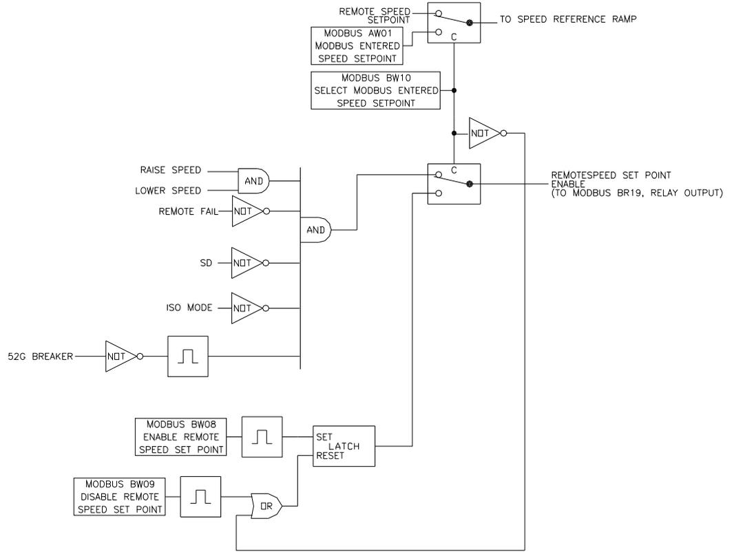
Figure 3-40. Remote Speed Control Setting
