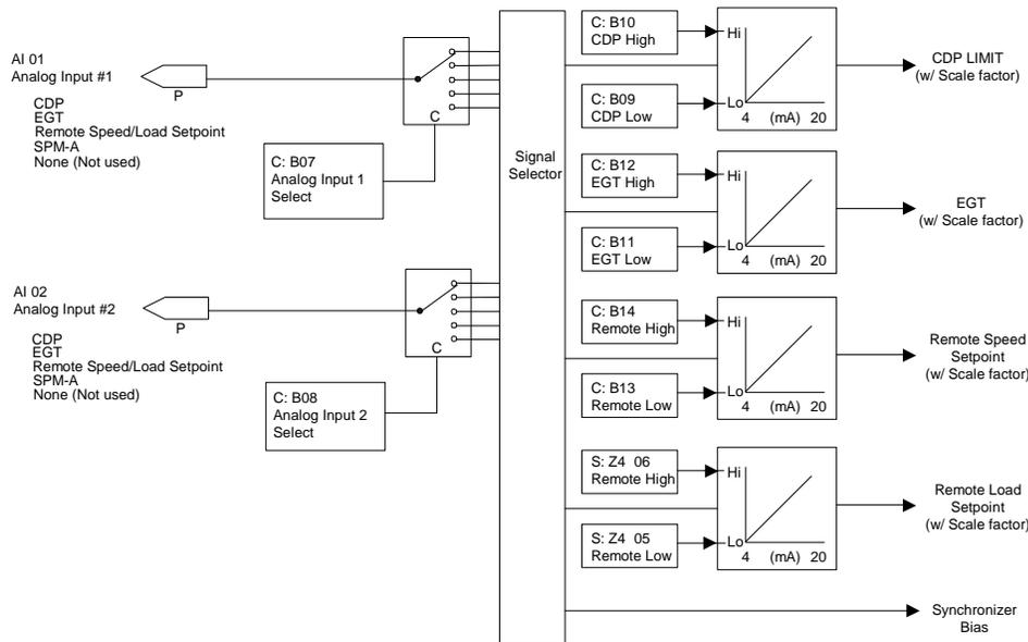
Figure 3-10. Selecting Analog Inputs
