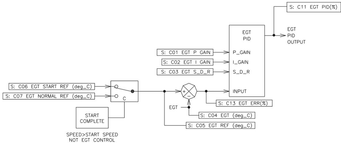
Figure 3-27. EGT PID SETTING
