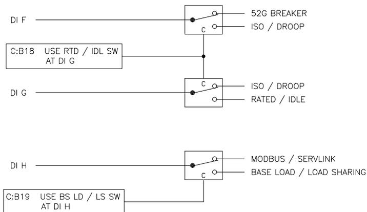
Figure 3-12. Discrete input Configuration
