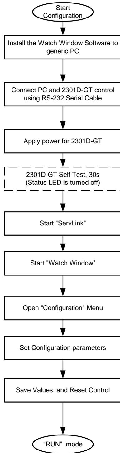
Figure 3-1. Basic Configuration Procedures
