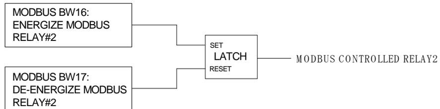
Figure 3-56. MODBUS CONTROLLED RELAY#2
