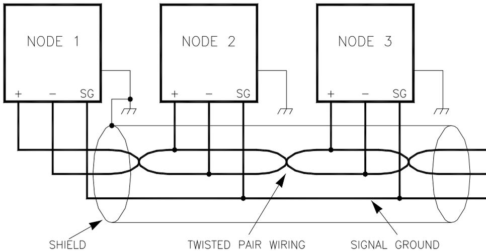
Figure 2-11. Preferred Multipoint Wiring Using Shielded Twisted-pair Cable with a Separate Signal Ground Wire
