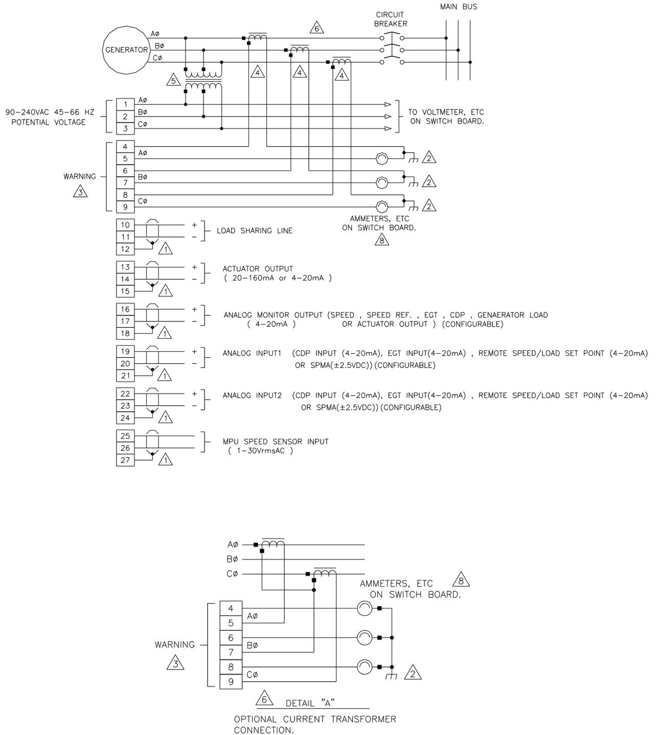
Figure 2-3. 2301D-GT Plant Wiring Diagram (sheet 1)
