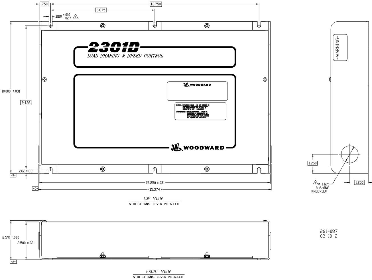
Figure 2-2. 2301D-GT P/N 8273-1002 Outline Drawing (hazardous location w/ external cover installed)
