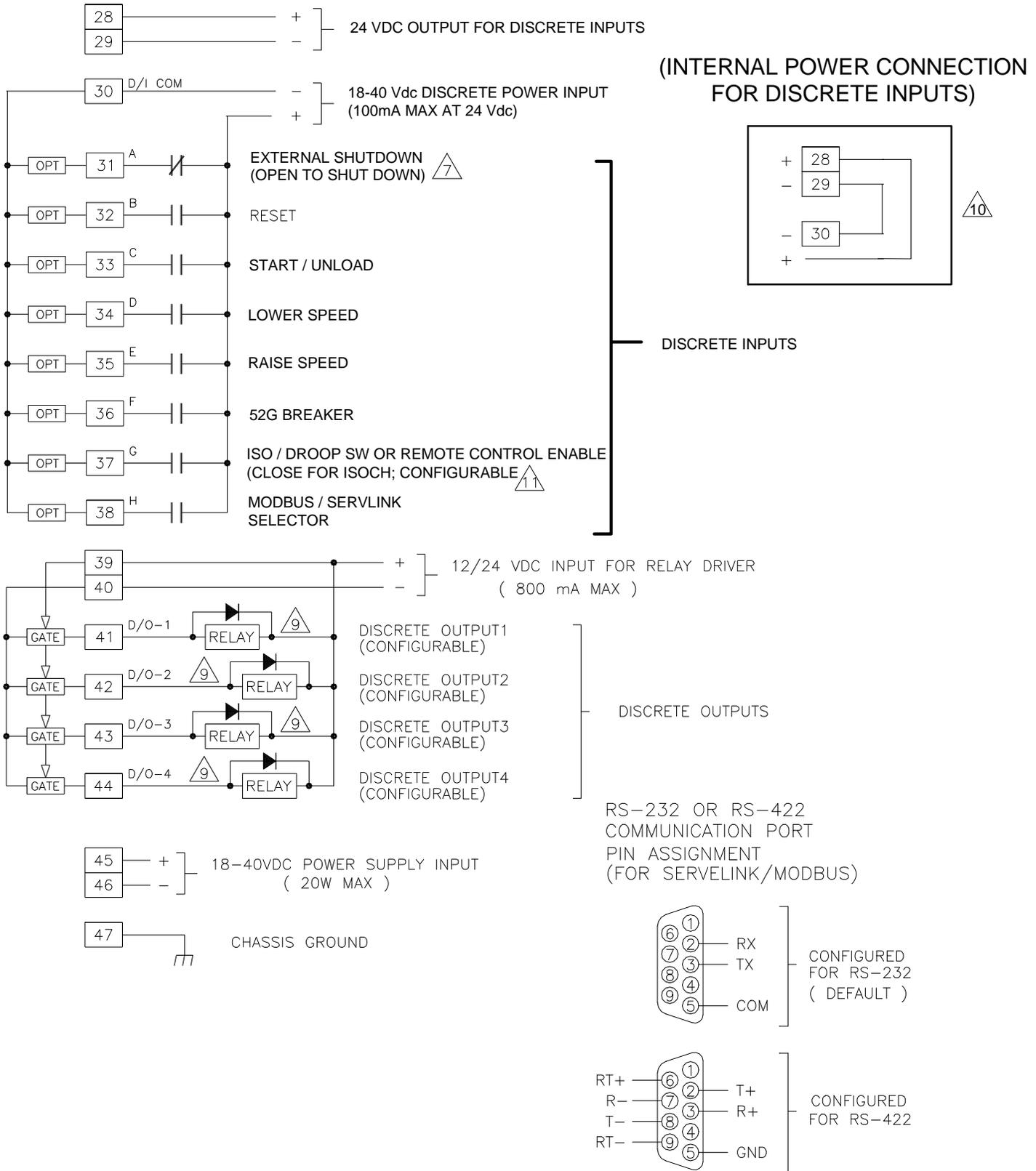
Figure 2-4. 2301D-GT Plant Wiring Diagram (sheet 2)
