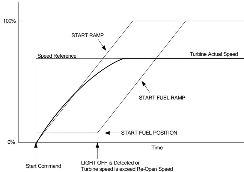
Figure 3-14. Unit Start Sequence Diagram
