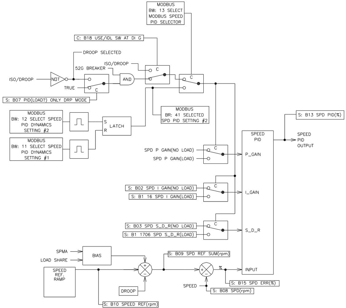
Figure 3-23a. SPEED PID SETTING1
