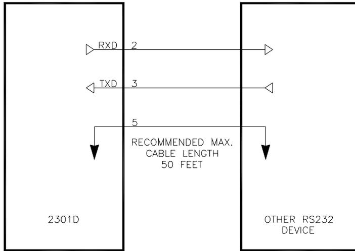
Figure 2-8. RS-232 Pin assignment for Serial Communication Cable
