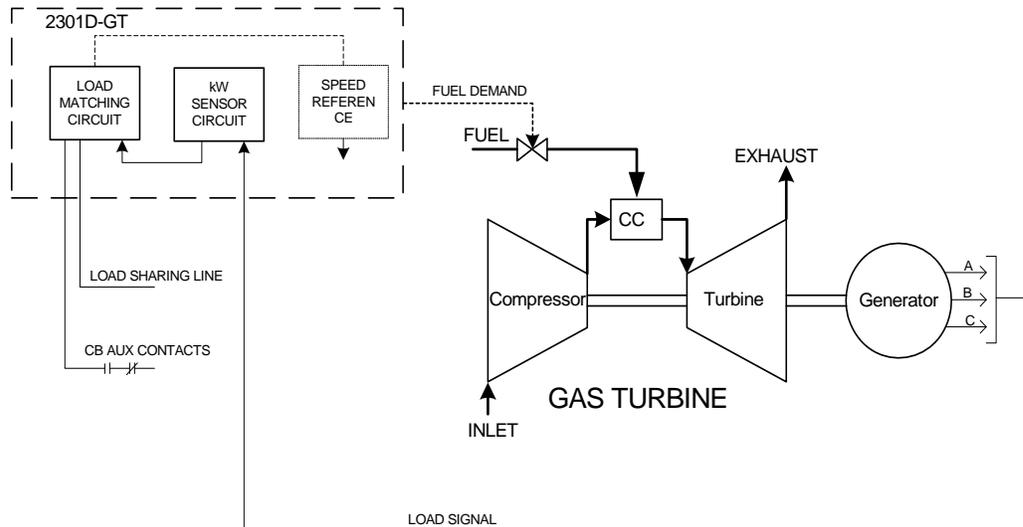
Figure 4-6. Paralleling System
