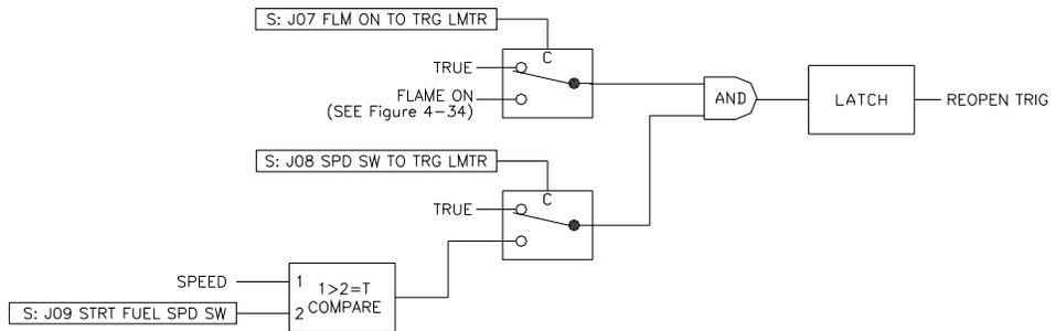
Figure 3-38. Start Fuel Ramp Setting
