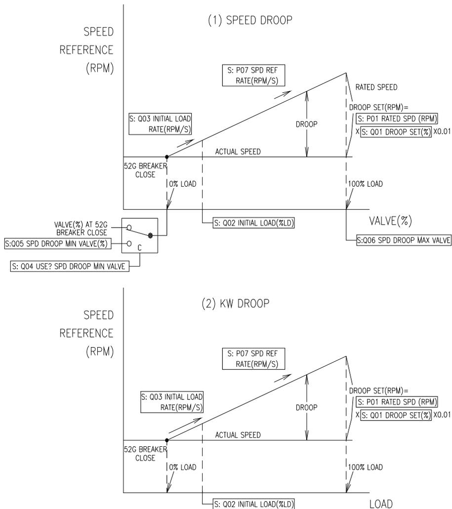
Figure 3-49. Load Control setting (Droop)
