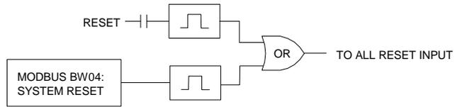
Figure 4-2. Reset Input
