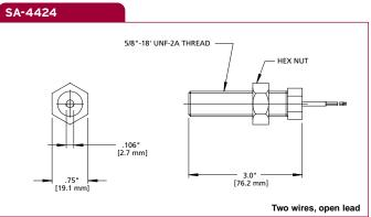
Use Woodward magnetic pickups with electronic speed switches for the input signal normally obtained from a gear tooth. Models SA-4423 and SA-4424 come with cable assembly for connection to the speed switch. For connection of Models SA-2170 and SA-2171A, cable lengths from 3 to 50 feet are available.
