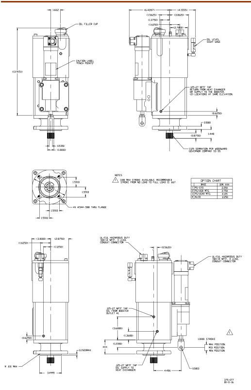
Figure 2-2. Outline Drawing of PGPL Actuator (12 ft-lb; spring return)
