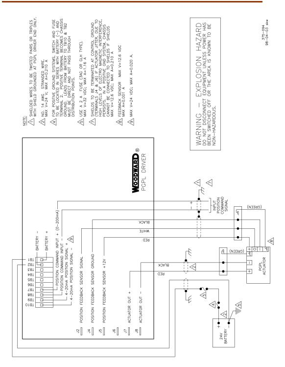
Figure 2-8. PGPL Driver Outline and Plant Wiring
