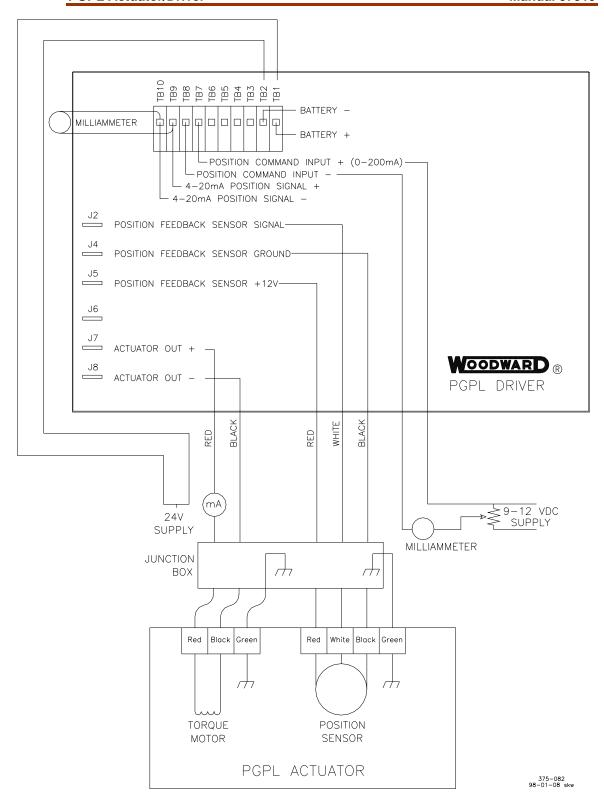
Figure 5-1. Test Wiring Schematic
