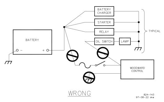
Figure 2-10. Wiring Direct from Battery to Control
