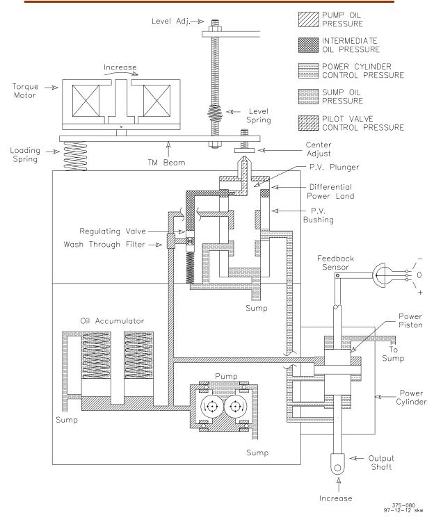
Figure 4-1. PGPL Actuator Schematic
